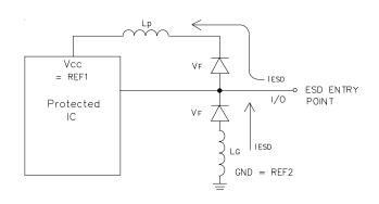
Figure 2 - The Effects of Parasitic Inductance When Using Discrete Components to Implement Rail-To-Rail Protection
