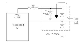
Figure 3 - Rail-To-Rail Protection Using RailClamp TVS Arrays
