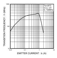
Fig.5 Gain bandwidth product vs. emitter current
