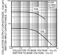
Fig.6 Collector output chapacitance vs. collector-base voltage Emitter input capacitance vs. emitter-base voltage
