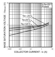
Fig.4 Base-emitter saturation voltage vs. collector current
