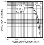
Fig.2 DC current gain vs. collector current
