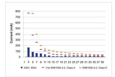
**Figure 3** — Typical input current harmonics, full load vs. V<sub>IN</sub> using typical applications circuit on pages 2 & 3
