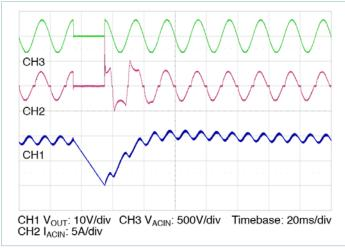
**Figure 11** — Line drop out, 90° phase,  $V_{IN} = 230V$ ,  $I_{OUT} = 8.3A$ ,  $C_{OUT} = 10,000 \mu F$
