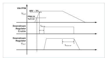
Figure 23 — PRM enable hold-off waveforms
