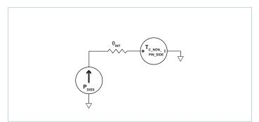
Figure 22 — Single-sided cooling thermal model
