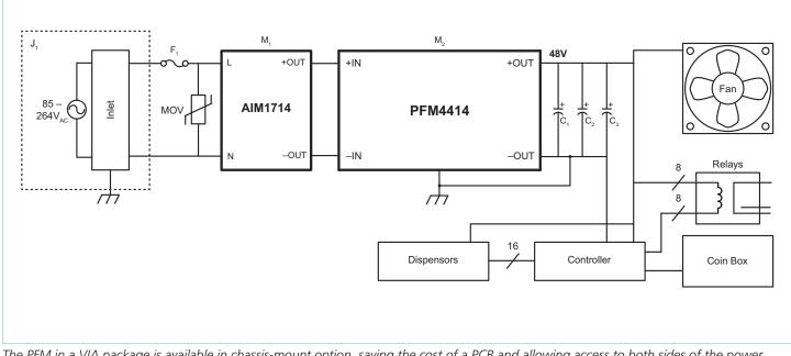
The PFM in a VIA package is available in chassis-mount option, saving the cost of a PCB and allowing access to both sides of the power supply for cooling. The parts list below minimizes the number of interconnects required between necessary components, and selects components with terminals traditionally used for point-to-point chassis wiring.
