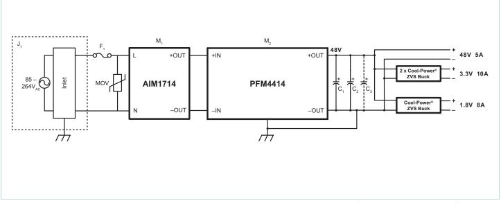
The PCB terminal option allows mounting on an industry standard printed circuit board, with two different pin lengths. Vicor offers a variety of downstream DC-DC converters driven by the 48V output of the PFM in a VIA package. The 48V output is usable directly by loads that are tolerant of the PFC line ripple, such as fans, motors, relays, and some types of lighting. Use downstream DC-DC point-of-load converters where more precise regulation is required.
