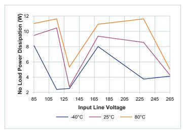
Figure 2 — Typical no load power dissipation vs. V<sub>IN</sub>, module enabled
