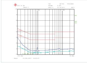
**Figure 13** — Typical EMI spectrum, peak scan, 90% load,  $V_{IN} = 115V$ ,  $C_{OUT} = 10,000\mu$ F using typical chassis-mount application circuit
