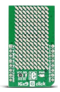
**16x9 G click** contains a **green LED matrix** and the IS31FL3731 audio modulated matrix LED driver. The dimension of the LED matrix is 16x9. Each LED can be controlled individually – both for on/off control and light intensity. The click is designed to run on either 3.3V or 5V power supply. It communicates with the target microcontroller over I2C interface and the following mikroBUS<sup>TM</sup> pins: PWM, INT, CS.
