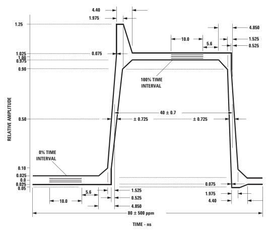
THE AFBR-5903 OUTPUT OPTICAL PULSE SHAPE SHALL FIT WITHIN THE BOUNDARIES OF THE PULSE ENVELOPE FOR RISE AND FALL TIME MEASUREMENTS.
