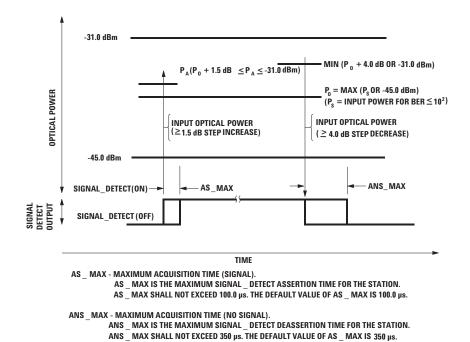
Figure 14. Signal Detect Thresholds and Timing.
