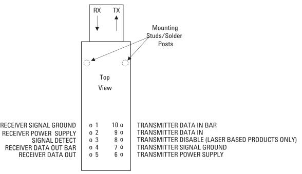
Figure 3. Pin Out Diagram.
