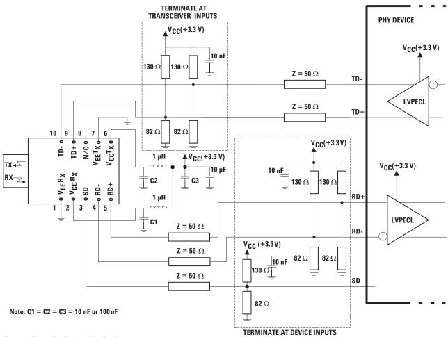
**Figure 8. Alternative Termination Circuits**
