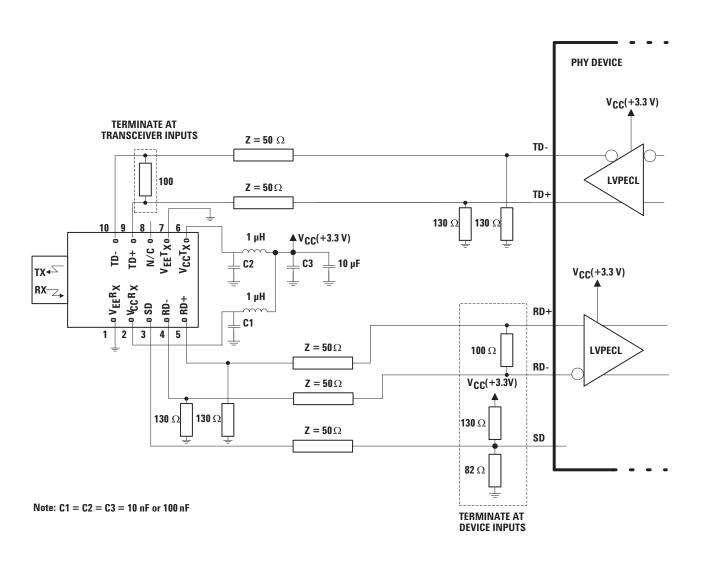
Figure 7. Recommended Decoupling and Termination Circuits
